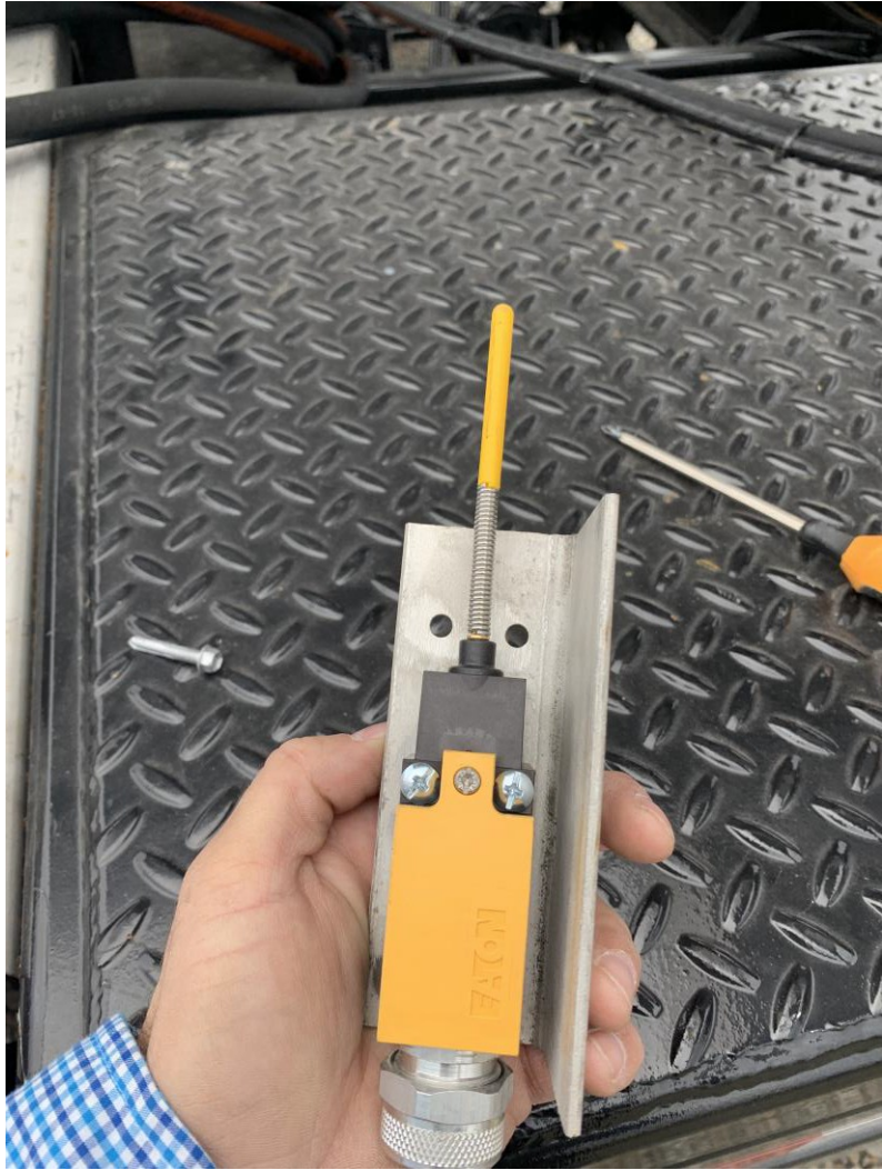
Step 5: Attach limit switch to mount as shown below with the limit switch mounting screws.
